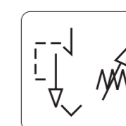
Pressure release valve
