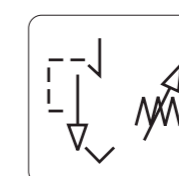
Pressure release valve
